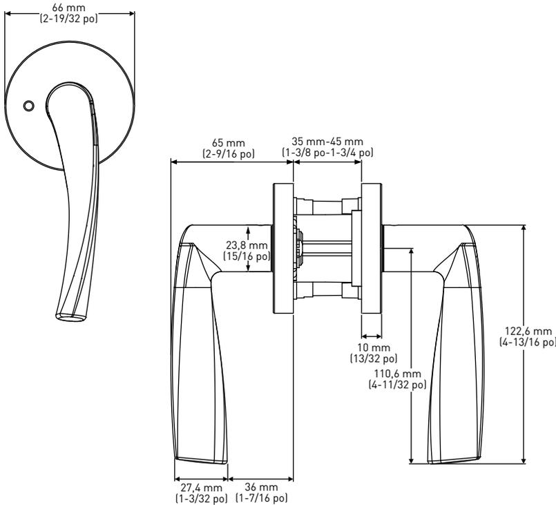
**LOQUET 6-EN-1 À ENFONCEMENT/À MORTAISE CARRÉE /À MORTAISE ARRONDIE À 45°**
