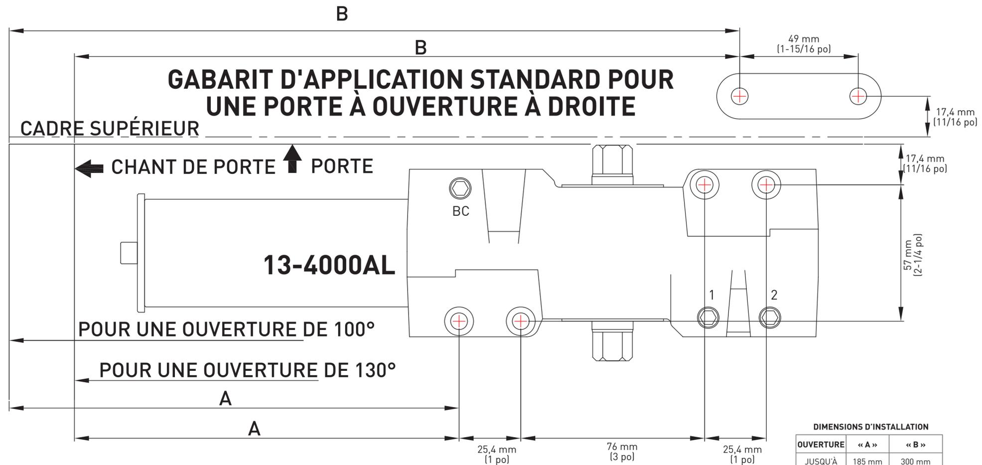
1 = VALVE/VIS DE VITESSE DE FERMETURE PRINCIPALE
