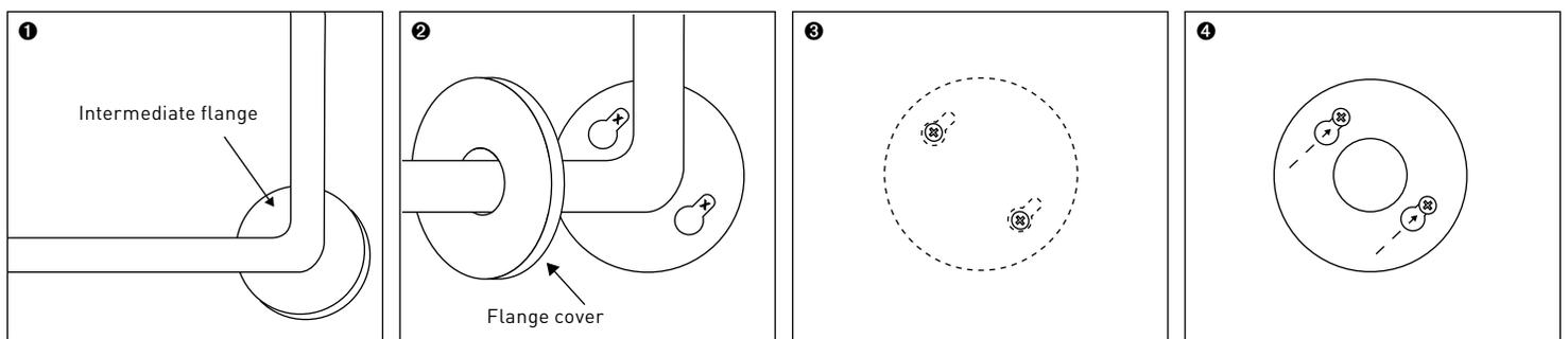
**1** Position the grab bar on the wall at the desired location. Use intermediate flange as a template to mark location of mounting screws for the intermediate flange only.
